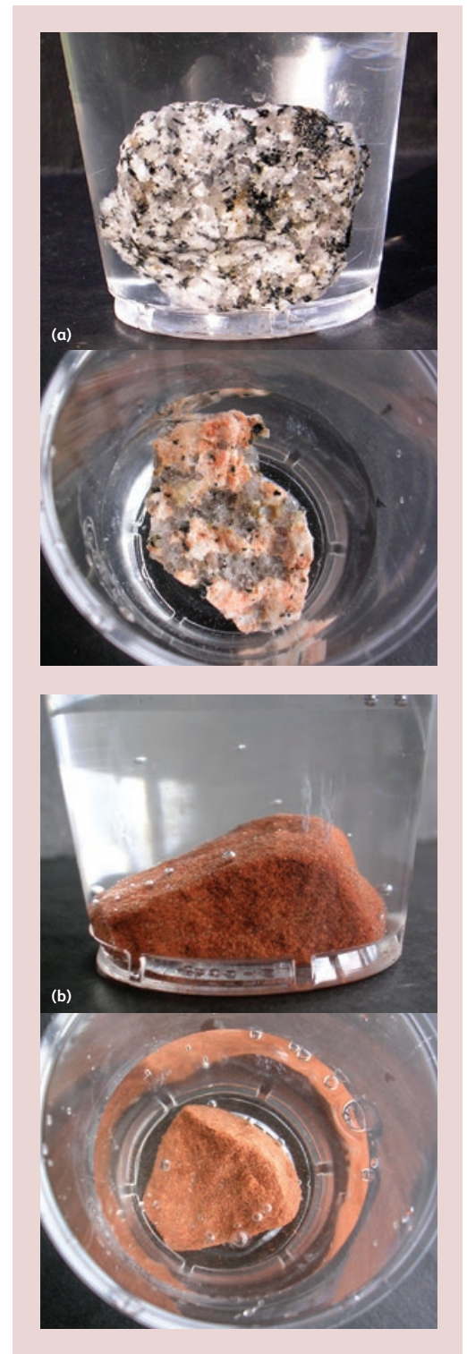
Figure 6: Rock types immersed in water to investigate differences in material grain arrangement – (a) granite (b) sandstone. Photos: © Peter Kennett/Earth Science Education Unit.
