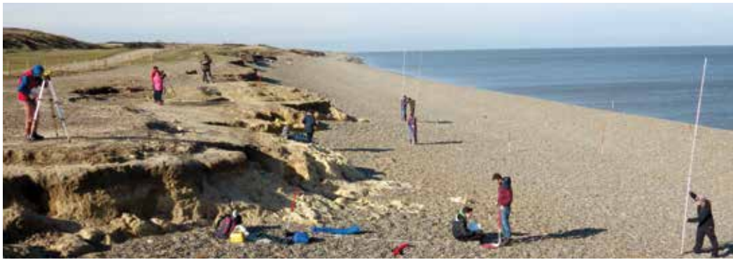
Figure 3: Students build up a bank of data by measuring from the same points each year. These measurements are used to monitor coastal change. Photo: Colin Bye.
