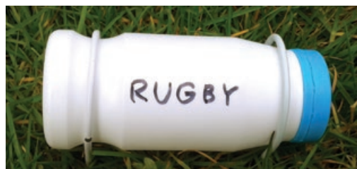
Figure 2: The small yogurt pot used to protect the logger from damp, pinned down to prevent removal. Photo: Geoff Jenkins.
