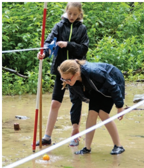
Figure 3: Students calculating velocity using a ranging pole, tape measure, stop watch and an orange. Photo: Rob Jones.
